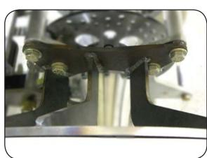
Note: side with more space from bolt holes to edge of fender goes toward the front.
