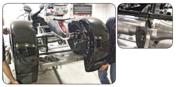
22. Torque fender bracket bolts to 60 ft. lbs.
