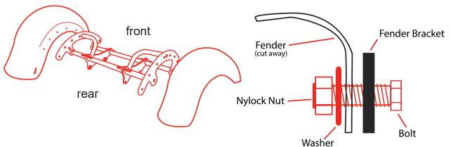
21. Remove two gold bolts on both sides. Install fender and bracket on the rear end.
