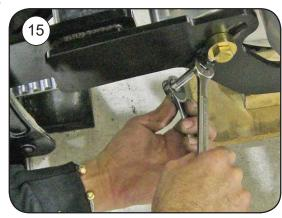
16. Torque the four rear end mounting bolts to 60 ft. lbs.
