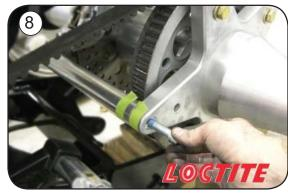
10. Install lower swing arm mounting bolts both sides, leave loose. Install upper swing arm mounting bolts, <u>make sure to put the 1/4" thick washer between the swing arm and the star plate on both sides,</u> leave loose. Refer to diagram for placement of washers and spacers.
